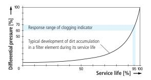
The dirt load collected in a filter element gradually increases during service, which also leads to a higher pressure drop. The resulting differential pressure  $\Delta p$  is monitored by a clogging indicator. Once a preset value is reached, an electrical and/or optical signal is generated. The following must be observed in this context:
