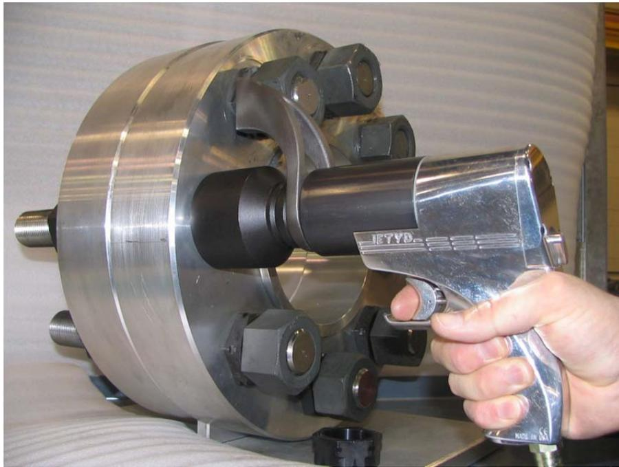
4. Ensure the torque wrench is set to the loosening direction.
