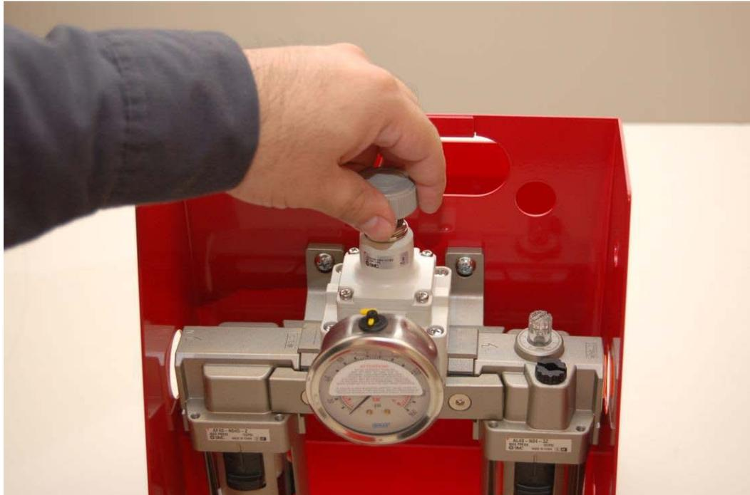
2. A Torque Chart is provided with each tool which gives the conversion from air pressure (PSI) to torque (ft-lbs and N-m). Use the chart to determine the air pressure needed to achieve desired torque output.
