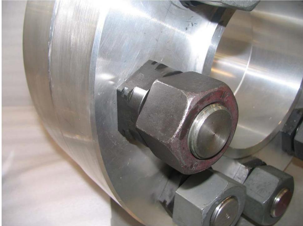
5. Install the lubricated nut by turning it clockwise down the bolt until it is firmly hand tight against the HYTORC reaction washer.
