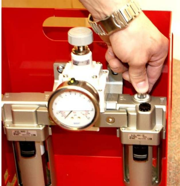
3. Turn the flow adjustment knob clockwise or counter-clockwise until the oil is dripping at a rate of at least one drop every ten seconds.
