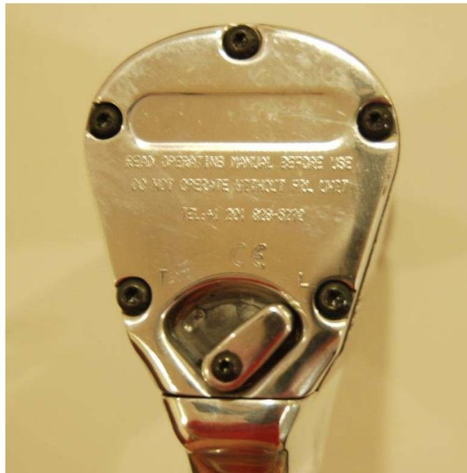
3. Be sure the lever is fully engaged in either direction before operating the gun.
