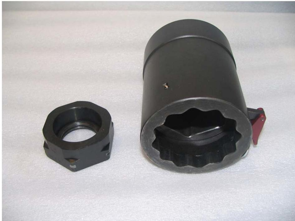
In addition to the added safety of having no external moving parts, the HYTORC Washer system provides a universal reaction point for all applications, eliminating the need for custom-designed reaction arms. Concurrently, the threaded segment inside of the washer stops the bolt from turning, eliminating the need for back-up wrenches. By reacting and tightening on the same axis, side-load is eliminated and surface friction from nut-to-nut is equalized, giving you increased bolting accuracy.
