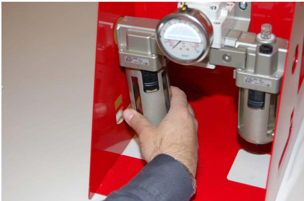
Figure 20. FRL Unit – Lubricator 2/3rds Full of Oil
