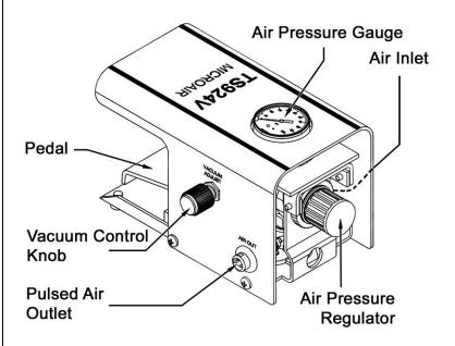
The TS924 Series dispenser is designed for use under the work bench. For this reason, a 6ft (1.8m) receiver head assembly should be used. The optional SH-300 syringe assembly stand makes the perfect accompanying bench holder.
