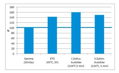
Structalit® 701 shows excellent bond strength retention after sterilization by autolaving, EtO and gamma irradiation. Generally the resistance depends on the substrate material, the curing parameters and the process of sterilization. It remains the user's obligation to determine the effect of sterilization on the specific procduct.
