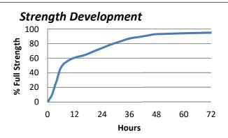
Graph shows typical strength development of bonded components at 23°C. An increase of 8°C in temperature will halve the cure time. Lower temperatures will result in a slower cure time.
