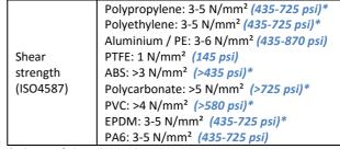
\*substrate failure observed
